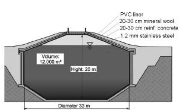
**Fig. 7** 12 000 m<sup>3</sup> hot water pit storage. Cross-section, main dimensions and components.
